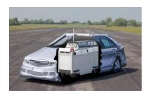
Advanced Driver Assistance System (ADAS) testing Guided Soft Target
