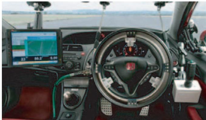
*Fig 4: Driverless Test System*
