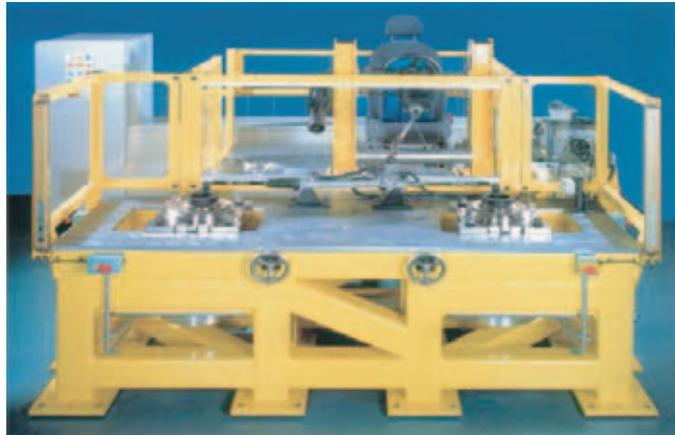
*Fig 2: Steering System Test Machine*
