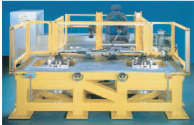
*Fig 2: Steering System Test Machine*
