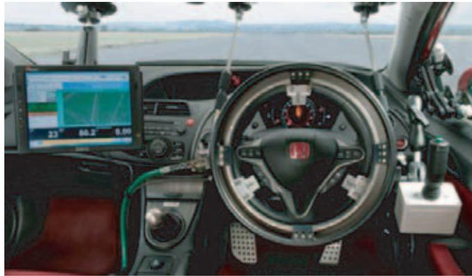
*Fig 4: Driverless Test System*
