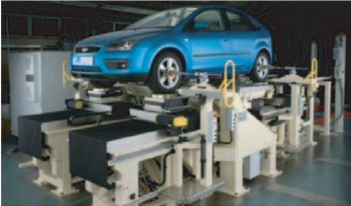
*Fig 1: Suspension Parameter Measurement Machine*
