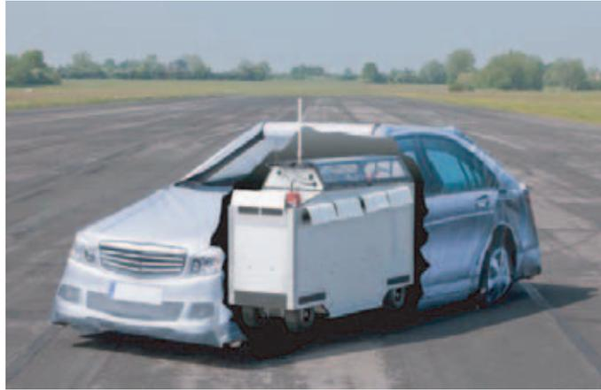
*Fig 5: Soft Crash Test Vehicle*
